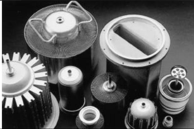
**Tube Bank.** ECONCO buys duds whenever possible for the purpose of having an inventory of the most commonly used types already rebuilt and in stock for delivery. The customer has the option to have a tube from stock (when available) or have a specific dud rebuilt.
