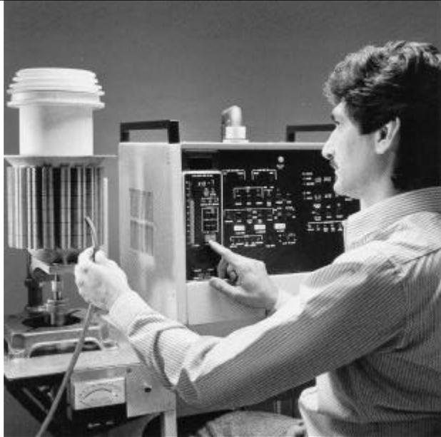
**Materials and Components.** Although ceramic has been replacing glass in power vacuum tubes, in many high voltage applications, glass is the preferred material. This tube has been opened on a glass lathe and is being prepared for rebuilding. Vacuum tube manufacture requires special materials and close-tolerance matching of parts. In the rebuilding process, all original tube specifications are met or exceeded.
