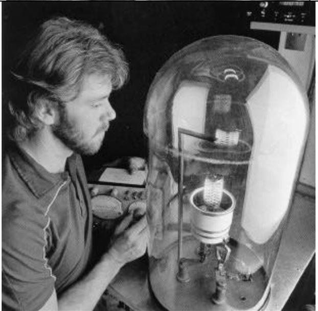
**Leak Detection.** Proper operation of a tube depends on a good vacuum within the envelope. The structure of the tube involves many different materials that are joined together. These joints must be vacuum tight. Here, seals are being checked on the mass spectrometer leak detector before further processing. The operational life of a tube is highly dependent on the degree of vacuum in the envelope; the better the vacuum, the longer the life.
