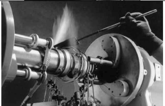
Tubes with cracked ceramics were previously considered unbuildable. Here, a 4CX3500A is prepared to have the cracked output ceramic removed and replaced.
